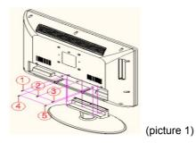
3. Using the plastic cover that came with the LCD screw in the 5 screws to fix the plastic cover on the bottom of the unit (Refer picture 2).
